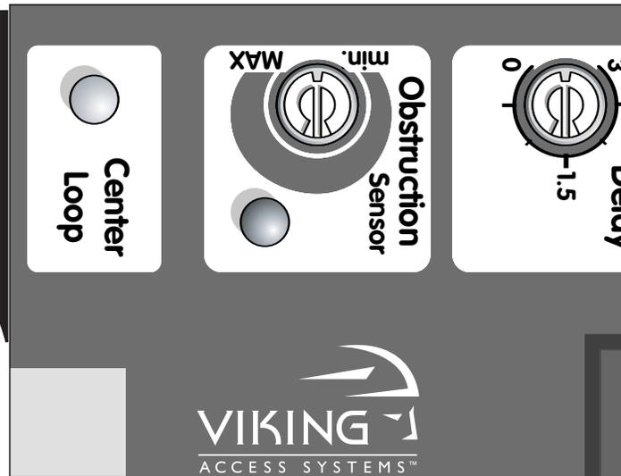
The Obstruction Sensor detects obstructions in the path of the traveling gate. The Trim Pot for the Obstruction Sensor adjusts the sensitivity level that triggers the Sensor.
