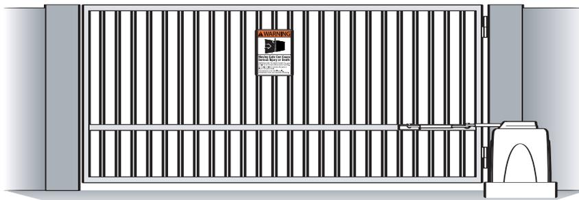
All Warning Signs and Placards must be installed where visible in the area of the gate. A minimum of two placards shall be installed. A placard is to be installed in the area of each side of the gate and be visible.
