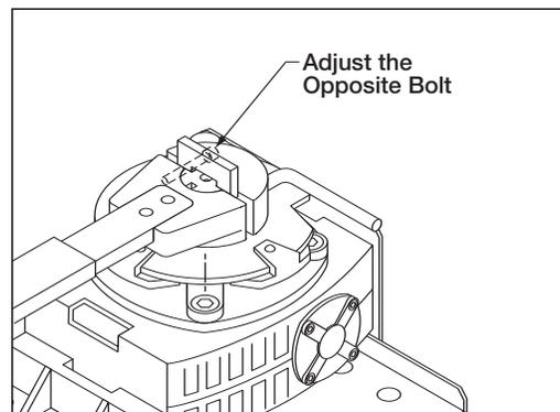
**NOTE** – For proper operation of the Clutch, keep the gap between the Clutch halves even when adjusting (the Clutch will have to be removed from the Output Shaft in order to adjust the Release Handle bolt).
