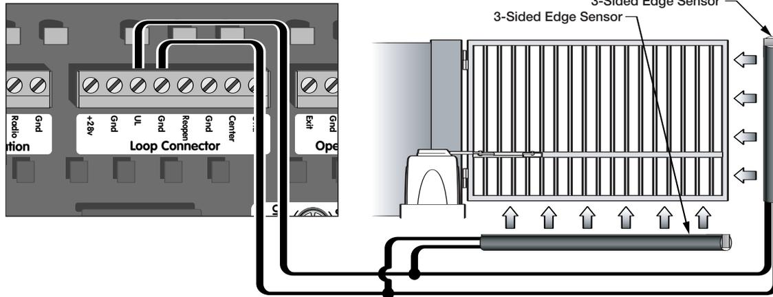
**Edge sensor or like must be installed to reduce the risk of entrapment.**
