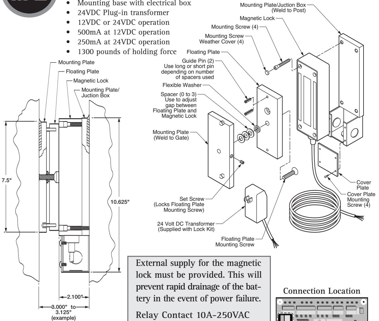
External supply for the magnetic lock must be provided. This will prevent rapid drainage of the battery in the event of power failure.
