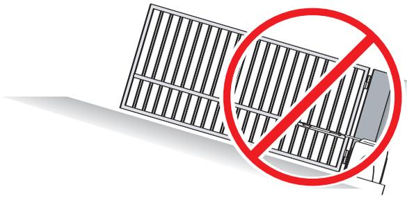
Do NOT Install the gate operator to lift gates
