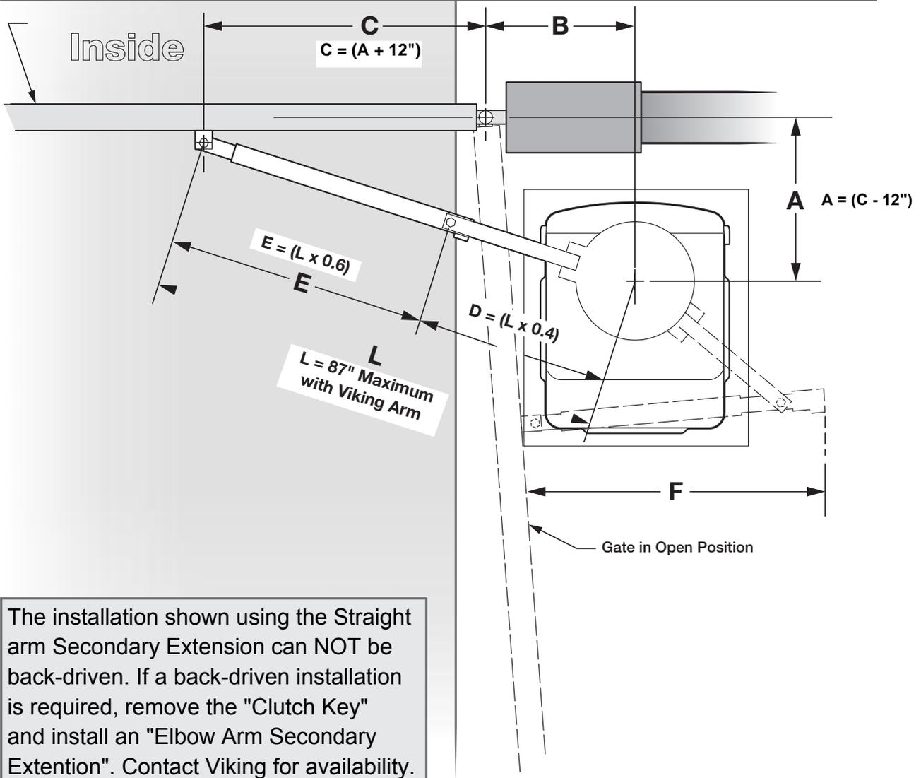
The installation shown using the Straight arm Secondary Extension can NOT be back-driven. If a back-driven installation is required, remove the "Clutch Key" and install an "Elbow Arm Secondary Extention". Contact Viking for availability.
