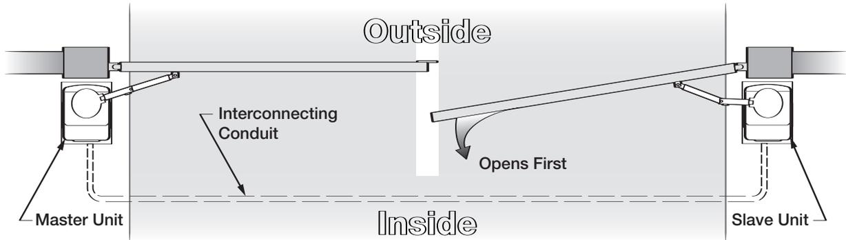
**Caution – Do not run Master/Slave communication cable in the same conduit as the power supply (120-220V) cable.**
