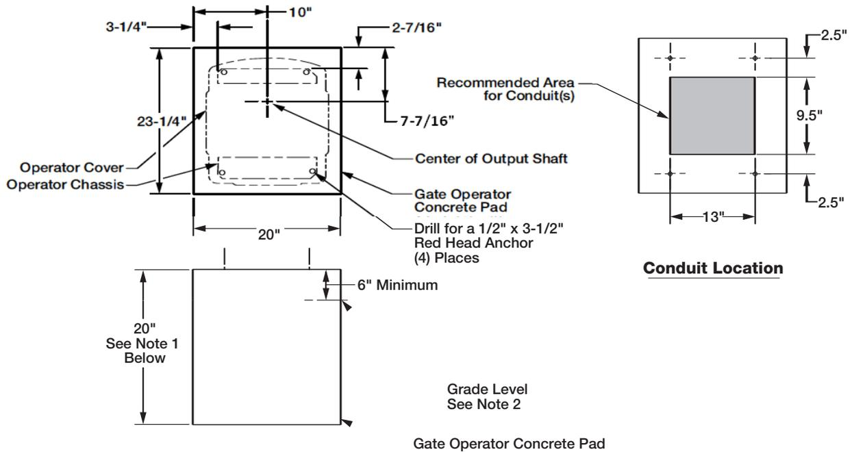
1. Follow the local building code to determine the required depth of the concrete pad.
