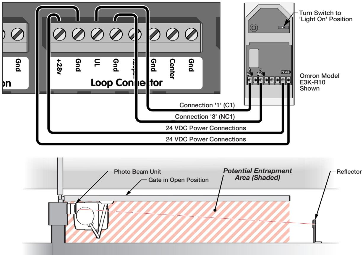
One or more non-contact sensors shall be located where the risk of entrapment or obstruction exists, such as the perimeter reachable by a moving gate or barrier.
