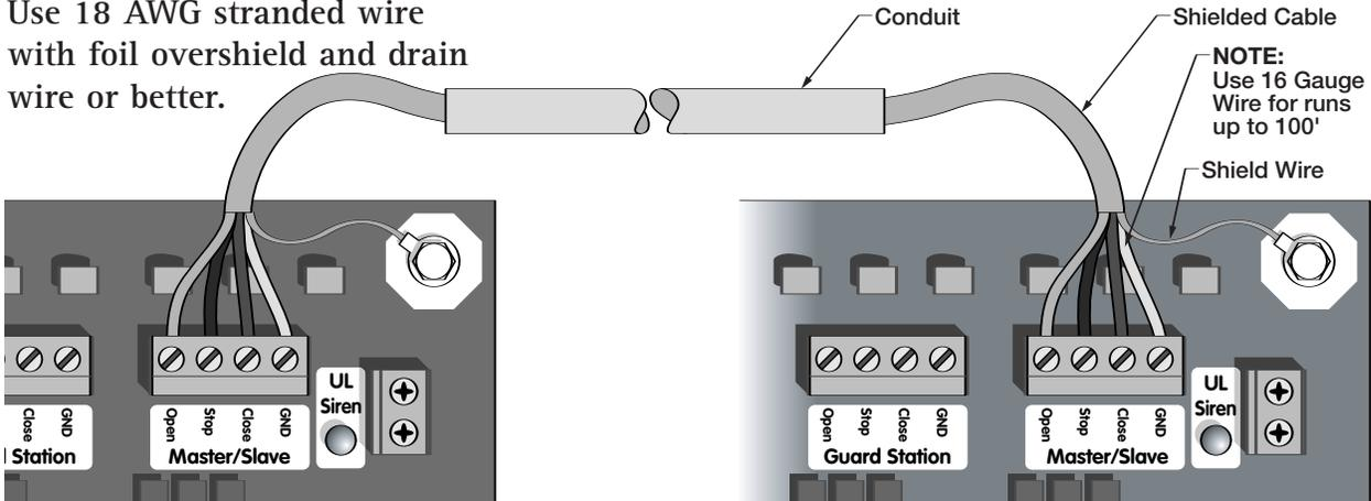
The control board provides a connector for master/slave connectivity. This connector will allow synchronized operation with a second gate operator.
